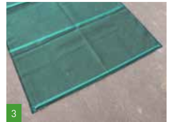
3 Start with group 1: lay a tarpaulin with the openings up and put the PVC pipe in the bottom hem, with the sleeve on the right.
