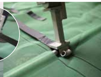
11 Use the stainless steel tensioner: place the base of the tensioner behind the steel tube where the tensioning belt is attached. Pass the belt through the opening of the tensioner. Pull the tensioner towards you and repeat. Do this for all belts. Re-tension 1 and 3 weeks after ensiling to compensate for silage compaction.
