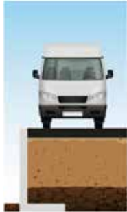
DLF10GS uniform distributed overload 25 kN/m 2
