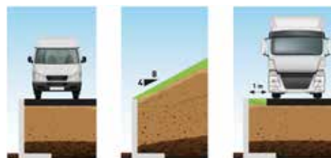
DLF10GS uniform distributed overload 25 kN/m 2
