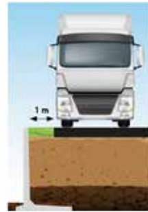
DLF10GSZ uniformly distributed overload 40 kN/m 2 at edge distance 1 m equivalent to load mode LM1 according to NBN EN 1991-2
