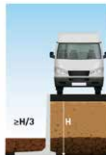
DLF10GSRZ uniform distributed overload 25 kN/m 2
