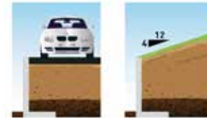
CLF10GS uniform distributed overload 10 kN/m 2 light traffic max. 3.5 tons
