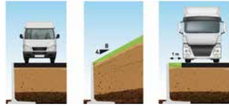
DLF10GSZ uniform distributed overload 25 kN/m 2
