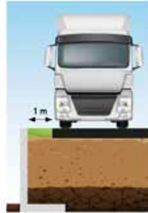
DLF10GS uniformly distributed overload 40 kN/m 2 at edge distance 1 m equivalent to load mode LM1 according to NBN EN 1991-2
